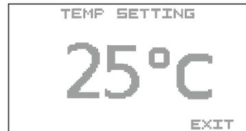
Applies to standard mode only. The choice of temperature - short press, exit - long press. Water spraying will be activated when this value is exceeded.
