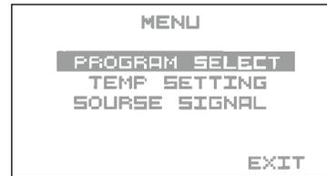
The menu is opened by long pressing the control button. Scroll - short press, select - long press.
