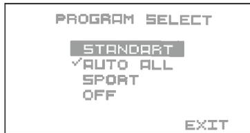
**STANDART:** Water spraying on the intercooler occurs when the intake air temperature and the load on the engine are higher than the values set by the user.
